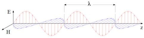
Figure 1. Electromagnetic wave (electric and magnetic field strength)
