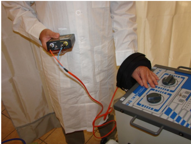
Figure 2. Measurement of electric current in upper limb of worker touching control panel of short-wave diathermy device generator with the use of clamp-on current meter
